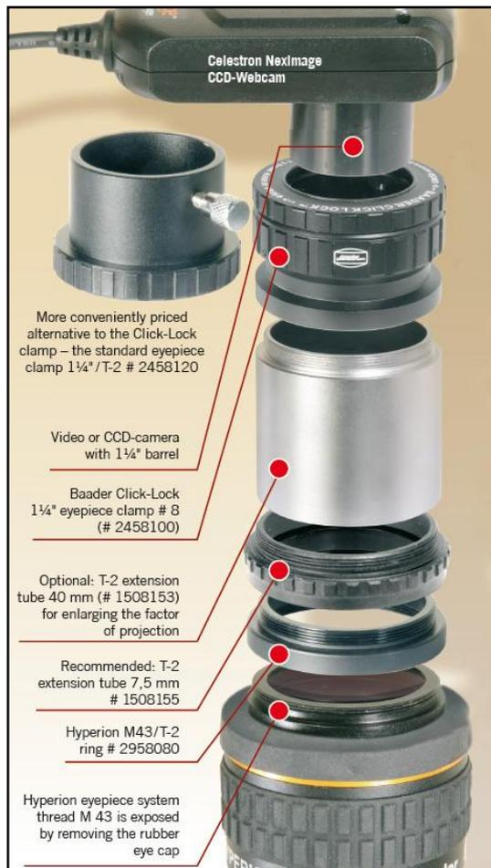
The illustration on the left side demonstrates a possible combination for classic eyepiece projection for webcams. Beginning at the bottom, the parts used a system thread M43 are:
