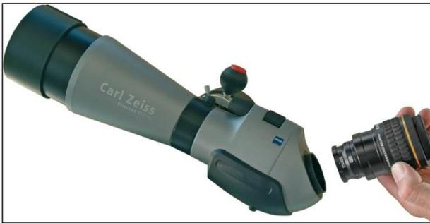
The 24, 21, 17, 13, and 8mm Hyperion eyepieces may be used with any Zeiss Diascope Spotting Scopes. A Baader Diascope bayonet eyepiece adapter 1¼" (#2454500) is required to attach 1¼" eyepieces to Zeiss Diascope Spotting Scopes. It is pushed onto the 1¼" barrel of the Hyperion eyepiece, and held in this position by three small locking screws locked against a bronze clamp ring that does not mark the eyepiece.
